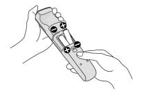
② Place two AA batteries in the remote control. Make sure that the batteries are properly oriented.
